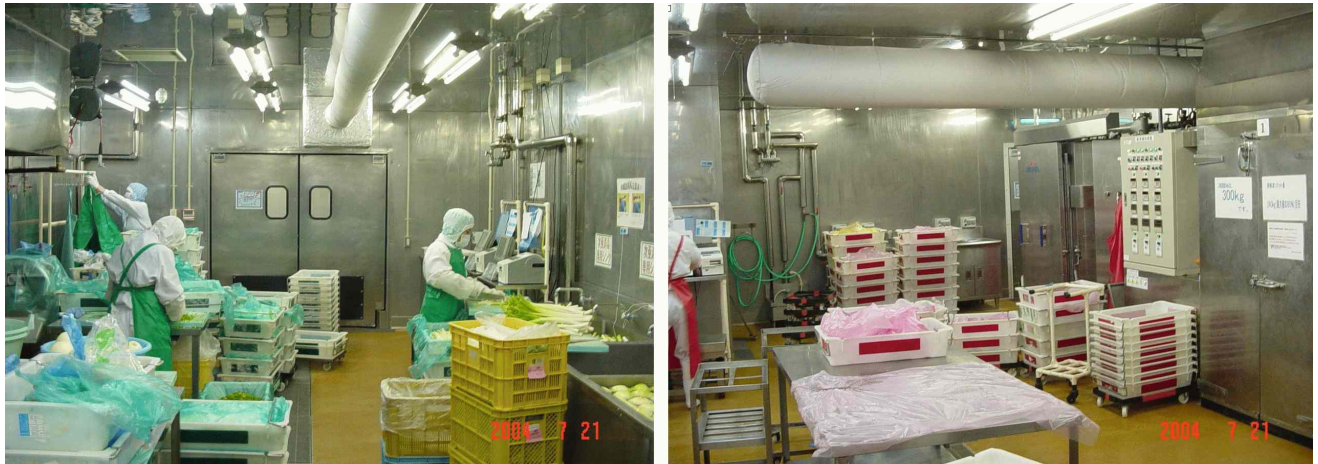
Figure 9: Blue (vegetables) and Red (chicken) coded bins in their respective preparation rooms.
